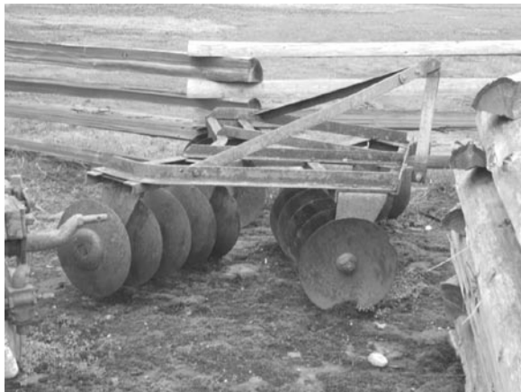
set of discs used for breaking up clods and preparing the soil for seed—Goat Farm
