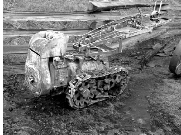
small tractor equipped for stump removal— Rowan Farm
