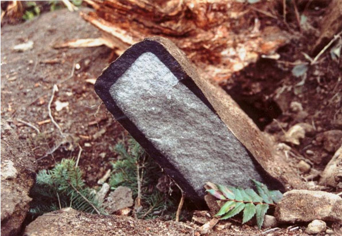
*Above:* A lovely example of “brown-stuff” weathering on a sandstone boulder freshly broken open during road construction in the interior of the island. A dark chocolate-coloured crumbly crust, 60-mm thick at its thickest, is covered by a thin outer veneer. The exposed inside of the boulder that we see here is slightly bluish-grey, typical for unweathered sandstone.
