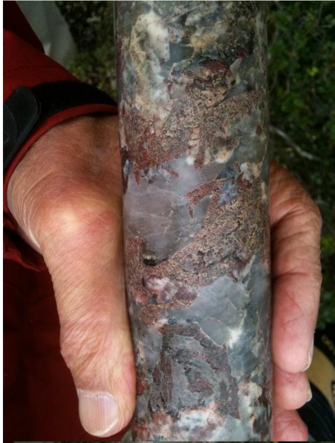
Figure 52: Diamond-drill granite core from the Strange Lake B zone. The deposit is unusually rich in rare HREEs.
